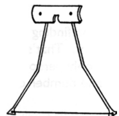
Another modification for mink. Hammer the ends of the trigger wires until they’re flat. Drill a 1/8” or 1/16” hole through each side. Tie a piece of 10-pound-test monofilament line between the holes.
