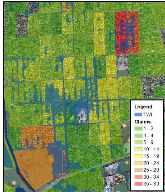
Figure F.11: Example of a topographic wetness index compiled for DuPage County. The index was overlaid with the claims per census block.
