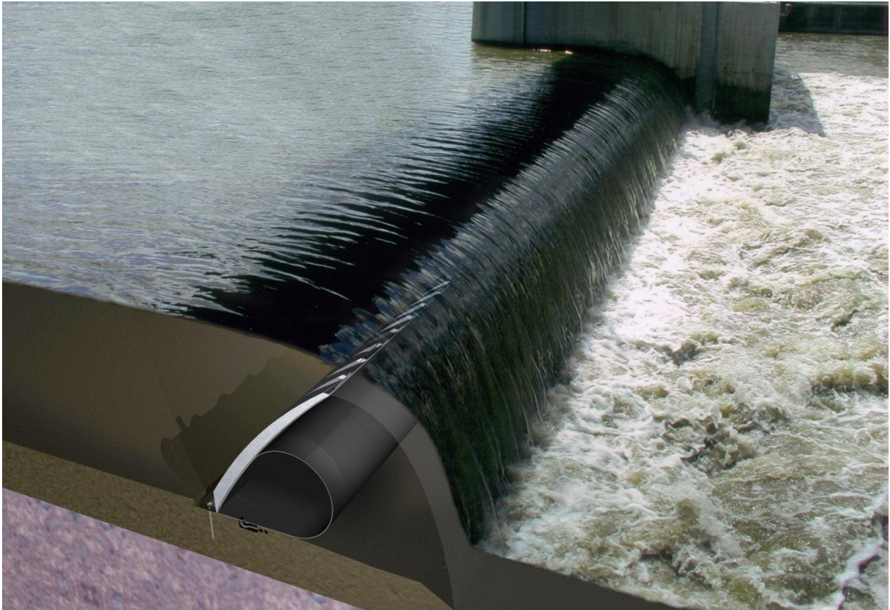
Figure 10: Cross Section View of Generic Hinged Crest Gate
