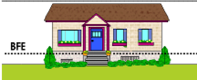
Figure 4. Same elevation crawlspaces
