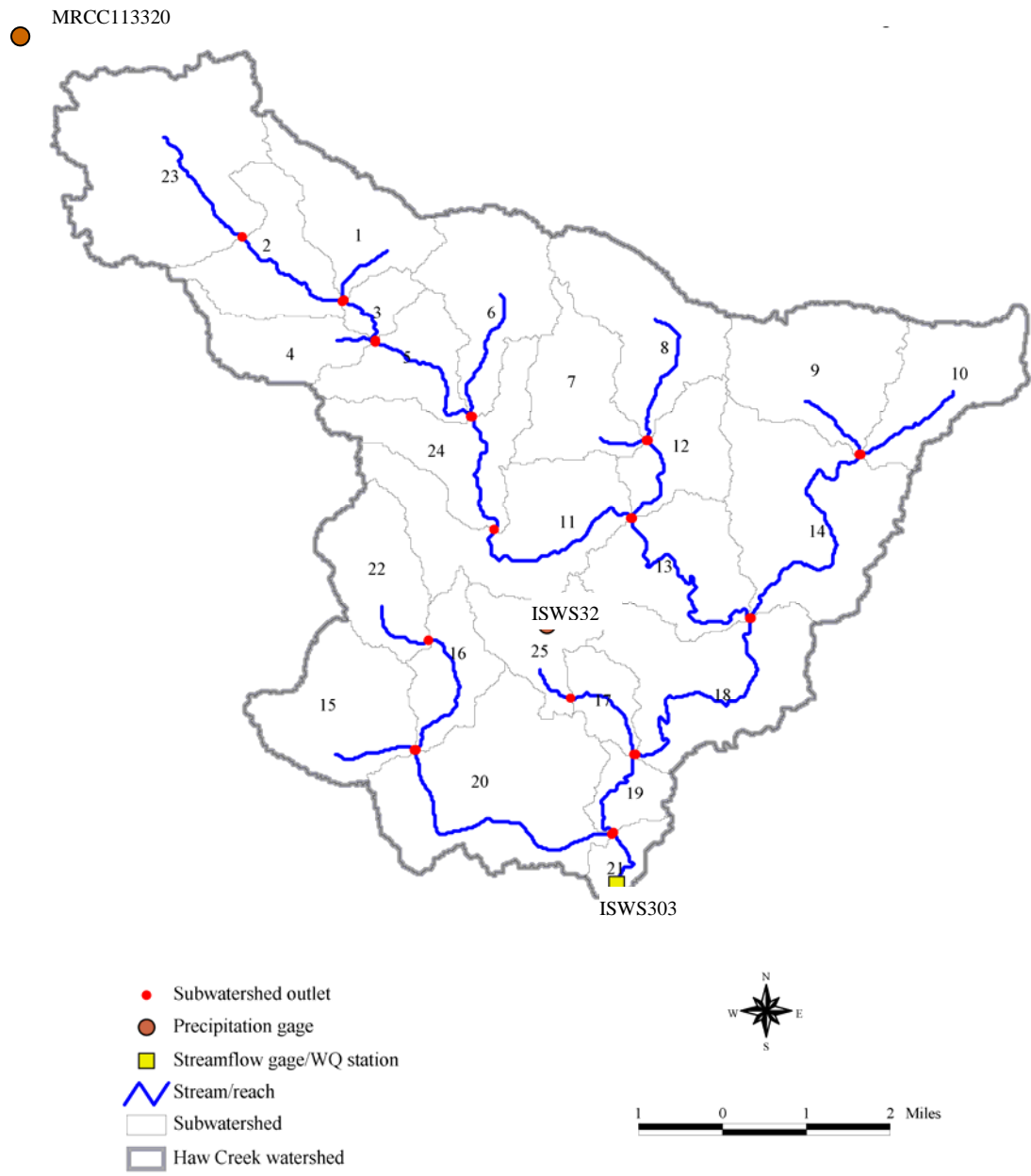
Figure 4-3. Schematic of the subwatershed and stream delineation, and precipitation gages used for the Haw Creek model
