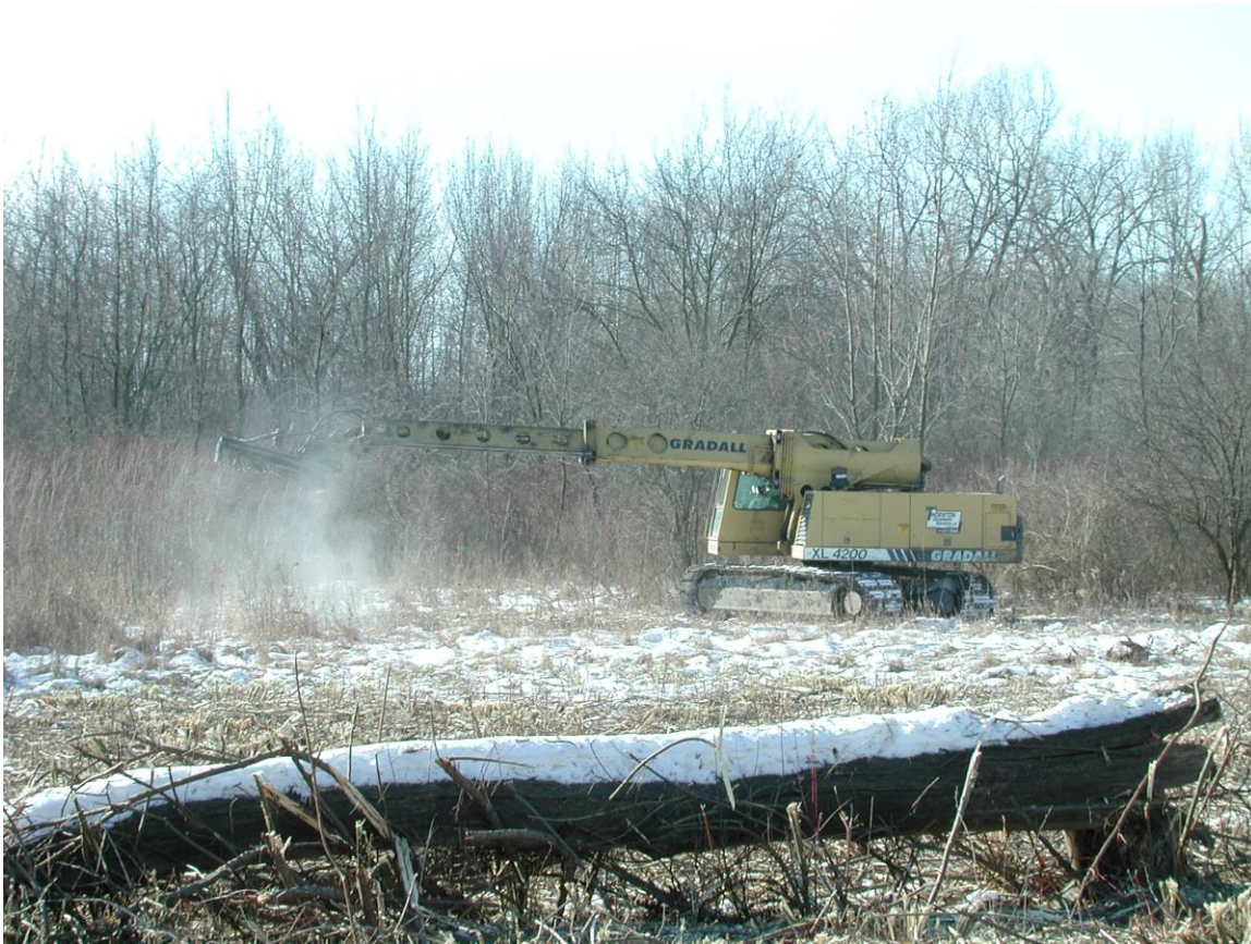
Figure C2. A forestry mower type head was utilized to remove exotic and invasive species at Wilmington Shrub Prairie in Will County. Follow-up herbicide treatment was completed.
