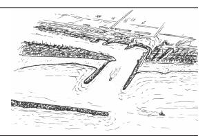
wing dam – man-made obstruction that extends into the river a certain distance instead of blocking the entire channel
