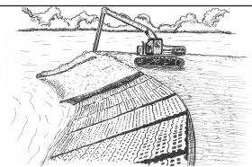
**jetty** – stone or dirt structure used to direct current or prevent shoreline erosion
