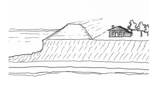
**revetment** – cement or wooden structure used to absorb the energy of the water and to prevent flooding and erosion
