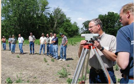
Wetlands expert Tom Biebighauser explains how basic survey equipment can be used to establish the proper elevations within seasonal wetlands.
