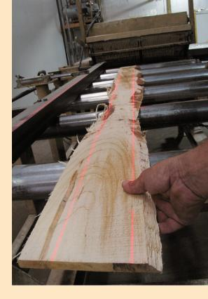
**Laser beams reduce waste for** precision cuts at a modern Illinois sawmill.
