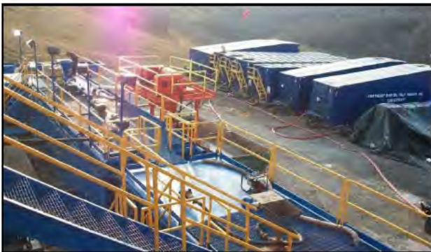
As an alternative to a lagoon, some drill sites use a series of frac tanks to collect flowback water.
