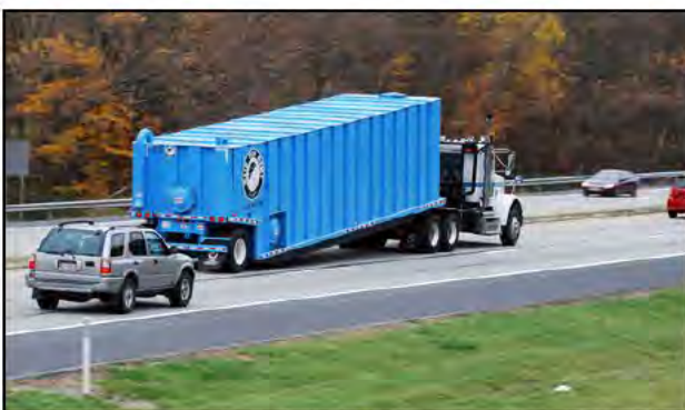
Frac tanks are hauled by trailer to a disposal location. Photo reprinted with permission of www.marcellus-shale.us .
