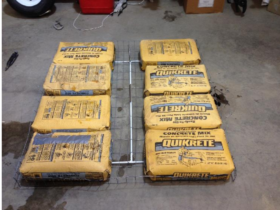
Digital Image 2. Concrete bags inside the frame & basket.
