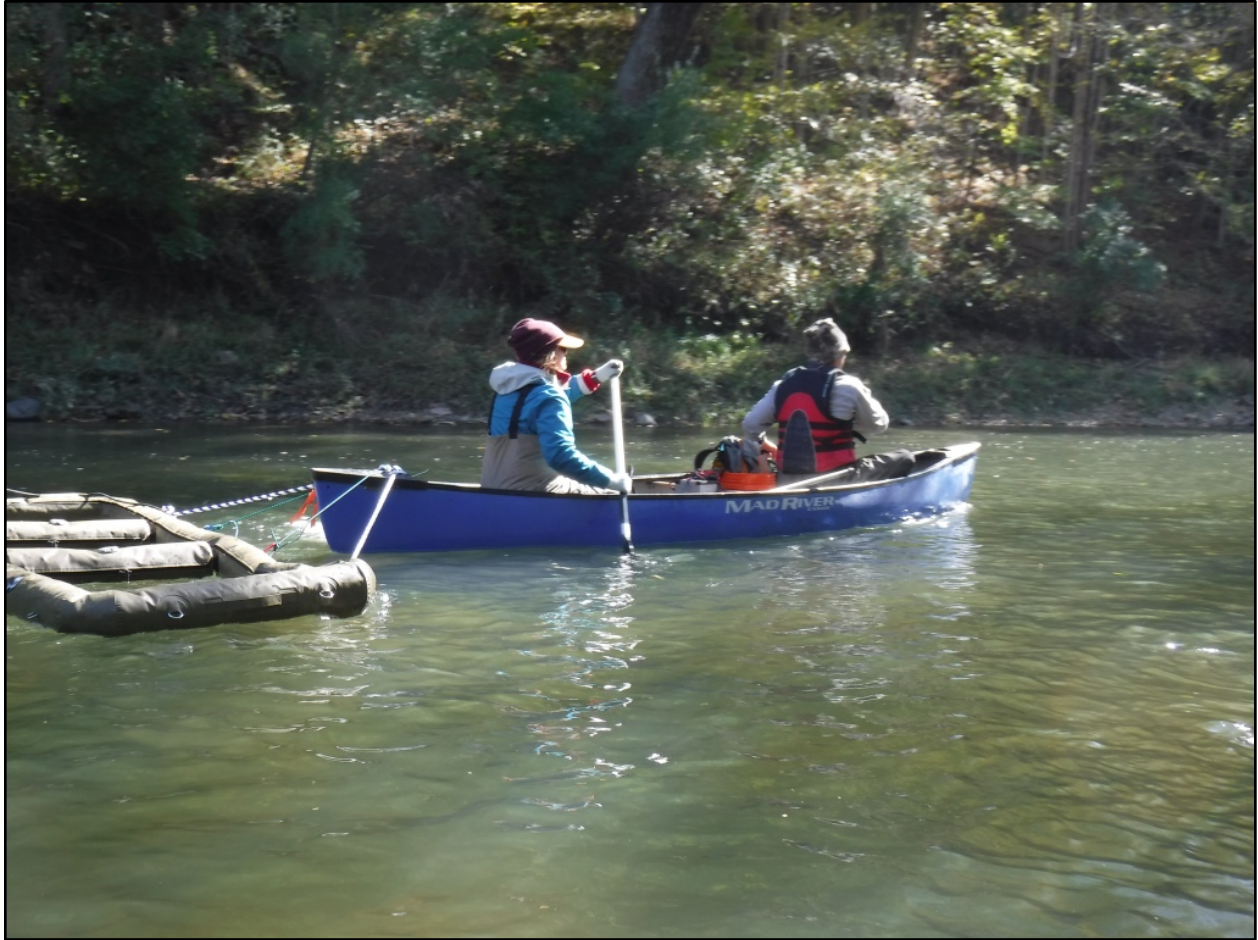
Figure 6. Researchers using a BioMark floating antenna to monitor PIT-tagged freshwater mussels. Pulling it behind canoe allowed INHS staff to cover vast distances not normally monitored, thus allowing researchers to encounter some translocated individuals >2 mi from where they were originally placed.
