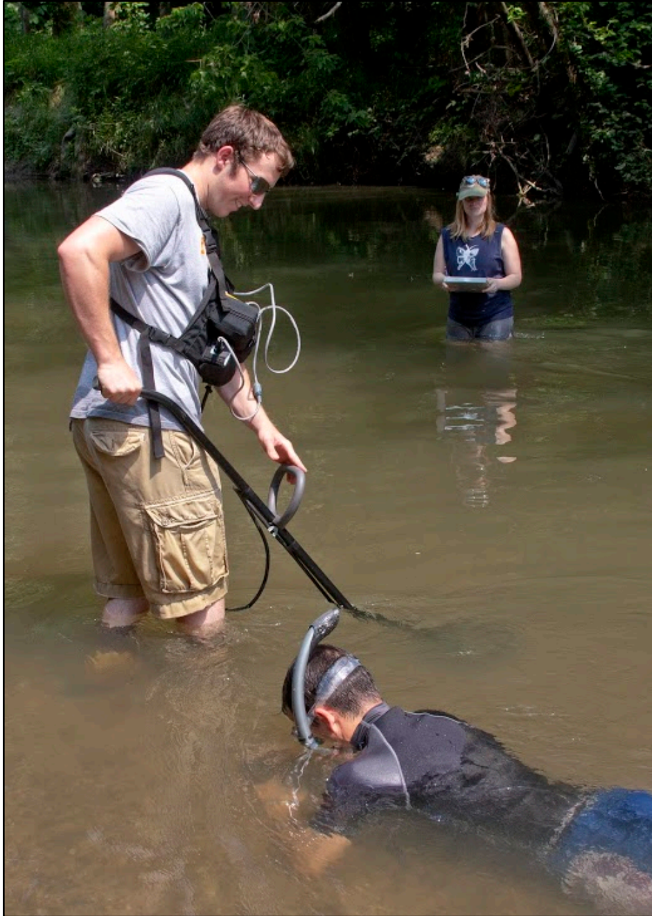
Figure 5. Researchers monitoring PIT-tagged freshwater mussels. When surveying for PIT-tagged mussels, a person carrying a PIT tag receiver wand slowly sweeps the streambed while walking the stream in a systematic manner. Detected tags are stored in the PIT reader, and data are later downloaded into a database after the sampling period ends. At least one additional sampler snorkels (or uses view buckets) if conditions are favorable and visually examines the streambed for tagged mussels. If an animal is seen, a note is made whether it was alive or dead. Photo courtesy of Rob Kanter (U of I).
