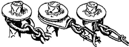
Left to right: lap-link, stake swivel and universal swivel.
