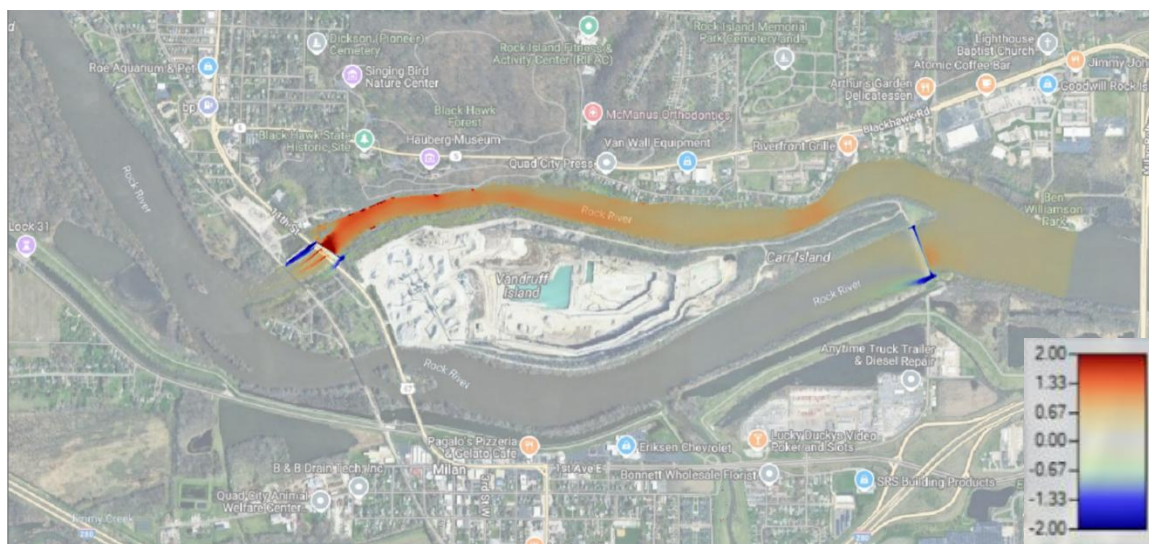
Figure 37: 15,500-cfs (Calibration/Max Recreation Flow) Change in Velocity-ft/s (Proposed Removal – Existing)
