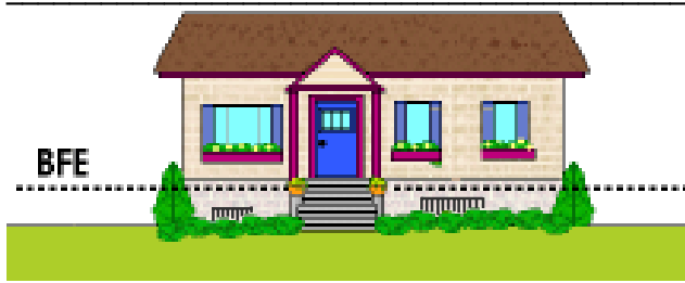
Figure 4. Same elevation crawlspaces
