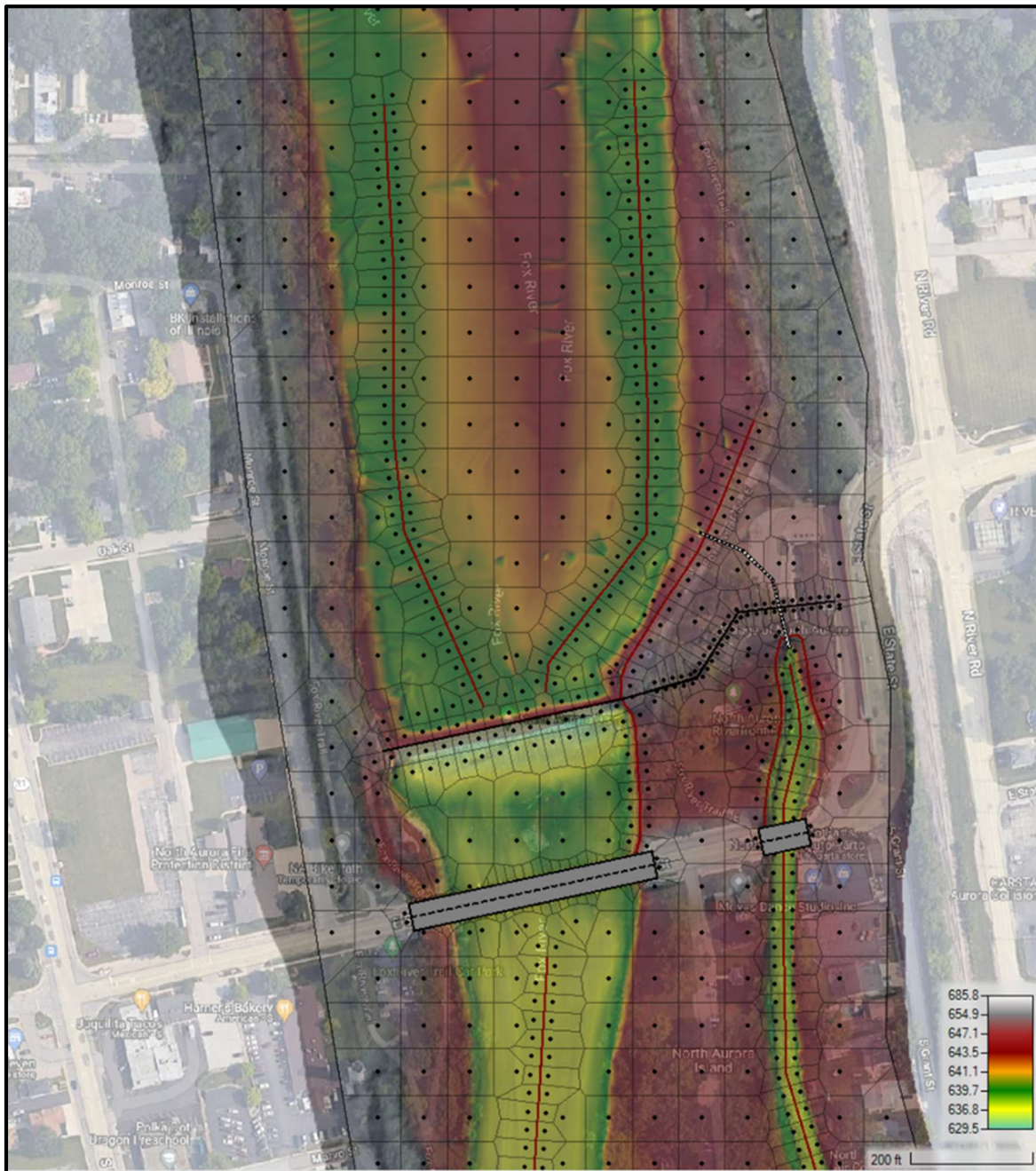
Figure 15. Closeup View of 2D Model Showing Cell Size
